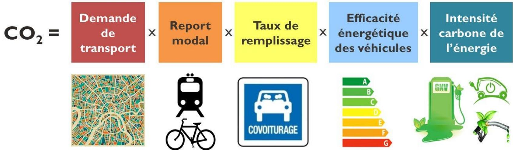
$$CO_{2,Transport} \equiv \sum_i D \cdot \frac{D_i}{D} \cdot \frac{C_i}{D_i} \cdot \frac{E_i}{C_i} \cdot \frac{CO_{2,i}}{E_i}$$
